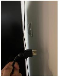
Image above showing the power plug on the unit which feeds from the back. Unplug this and plug back in to hard reset the system.
